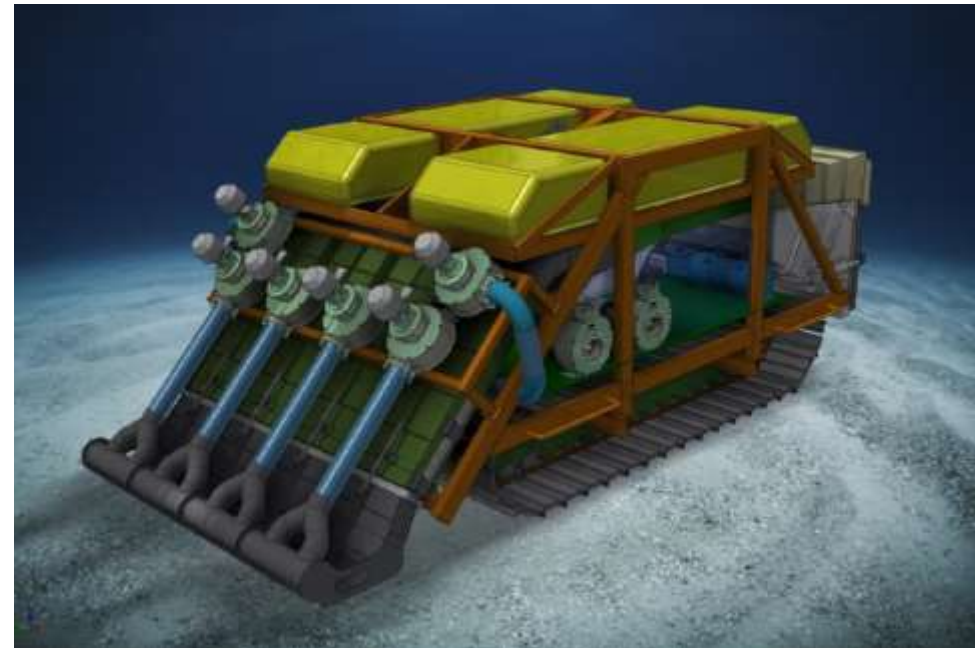
Prototype collector vehicle with 4-m wide collector head and tracked propulsion system; anticipated collector speed: 0.3-0.5 m/s
