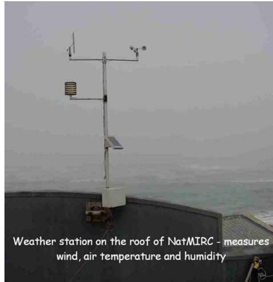
Figure 7. The weather station on the roof of NatMIRC in Swakopmund (photo taken by Deon Louw).
